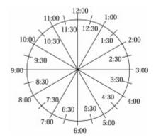
Holes should be located in degrees or clock time if possible, this will allow for the correct placement of holes. *Note: Every minute on the clock is*  $6^{\circ}$ .
